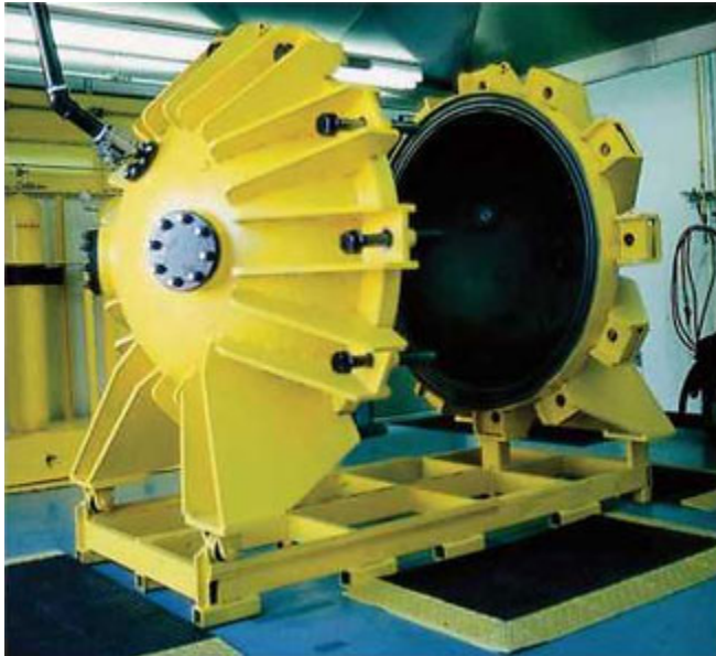
Test chamber used for standard explosibility testing (Fike-Corp.)
