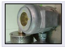
Totally-enclosed, fan-cooled (TEFC) explosion-proof motor in an electric explosion-proof / dust ignition proof vacuum cleaner.
