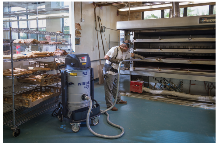
Hot oven cleaning with Nilfisk S2 industrial vacuum equipped with a Nomex filter and hot oven accessory kit
