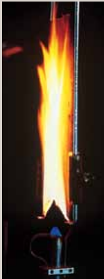
Vertical flame test on non-flame resistant fabric
