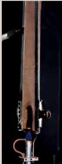
Vertical flame test on UltraSoft® fabric
