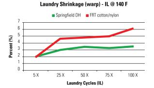
Springfield DH demonstrates several performance advantages over the compared FR treated cotton/nylon. Besides excellent wash and wear performance, the fabric has a low propensity for surface pilling due to its construction and finishing techniques. Union dye shades can be achieved with good colorfastness properties, an advantage over other blended fabrics. Hi-visibility shades are possible as specified by ANSI 107 and CAN 796.
